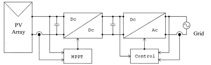
Fig. 13. Experimentally tested grid connected PV system.
