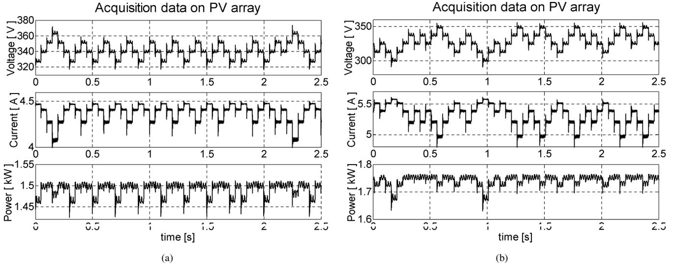
Fig. 14. Experimental measurements: (a) clear day and (b) cloudy day.
