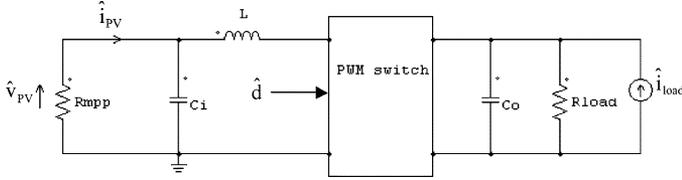
Fig. 5. Small signal equivalent circuit.
