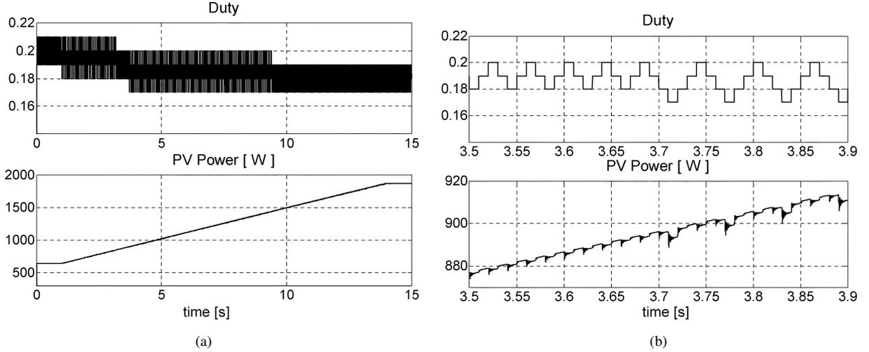
Fig. 10. Simulation results for:  $T_a = 0.01$  s;  $\Delta d = 0.01$ ;  $\dot{s} = 50$  W/(m<sup>2</sup>s); (b) zoom of (a).
