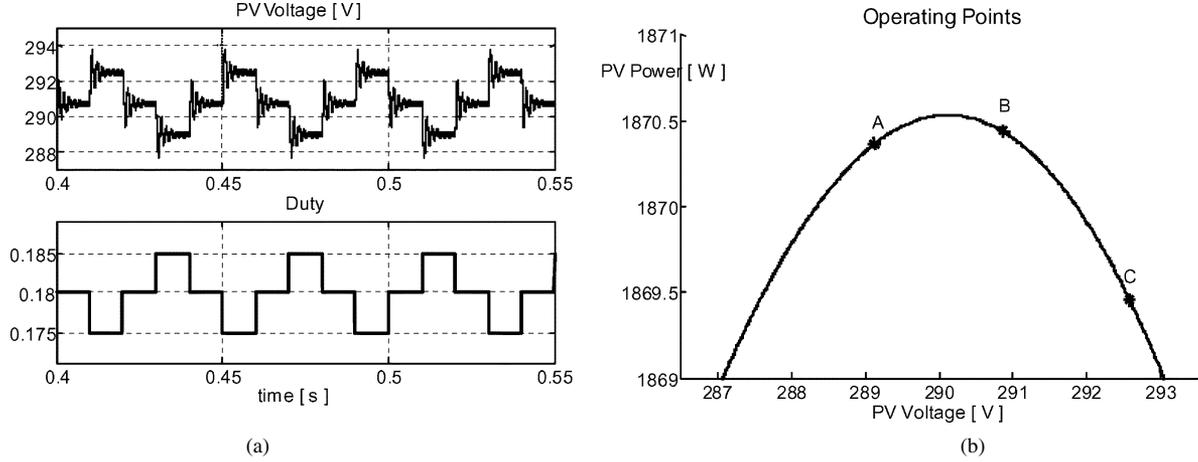
Fig. 7. Simulations with:  $\varepsilon = 0.1$ ,  $T_a = 0.01$  s,  $\Delta d = 0.005$ ,  $S = 1000$  W/m<sup>2</sup>: (a) time domain waveforms and (b) operating points location on PV characteristic.
