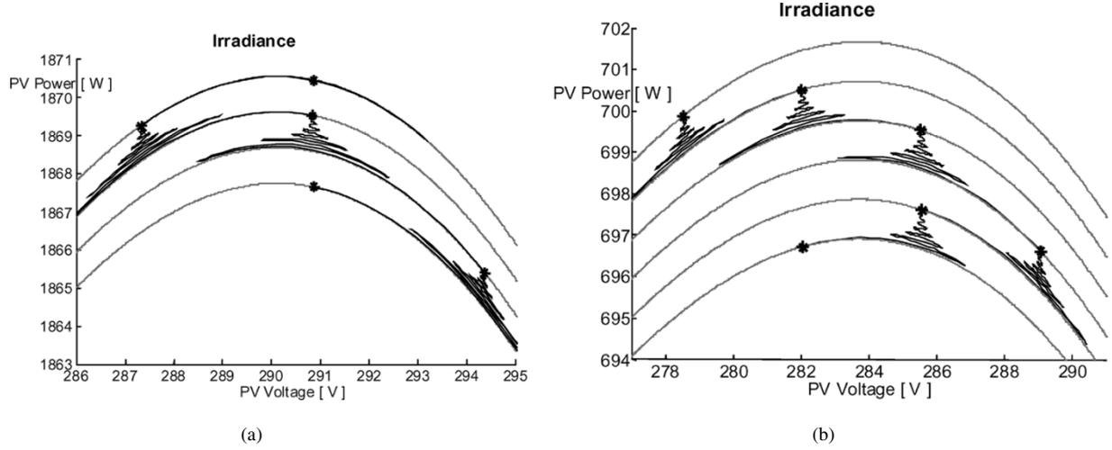
Fig. 11. Operating point of PV battery charger with  $T_a = 0.01$  s;  $\Delta d = 0.01$ ;  $\dot{S} = 50$  W/(m<sup>2</sup>s): (a) three points behavior and (b) four points behavior.
