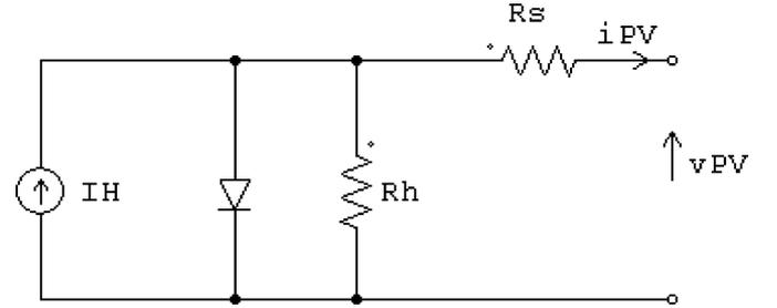
Fig. 4. Equivalent circuit of a PV array.
