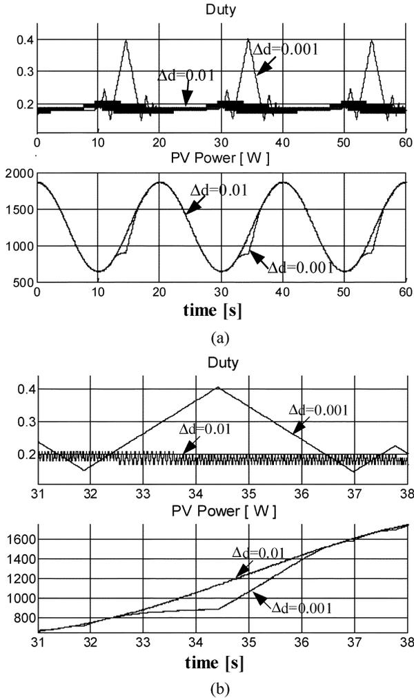
Fig. 12. Time domain simulations: (a)  $T_a = 0.01$  s;  $\dot{S}_{\max} = 50$  W/(m<sup>2</sup>s) and (b) zoom of (a).
